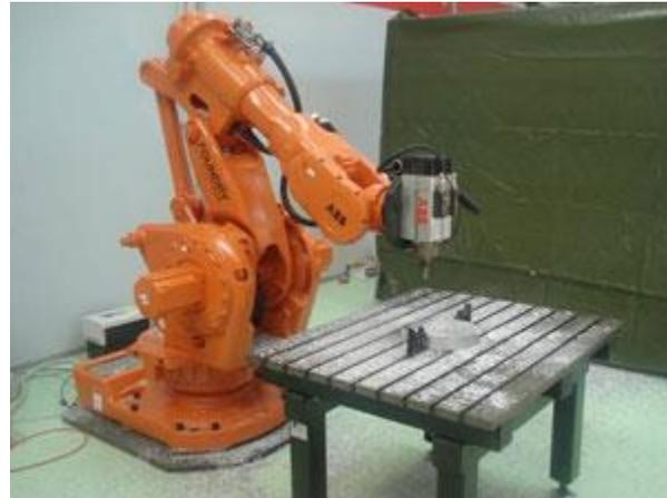
**ABB IRB6660 Robot Milling Aluminum**
