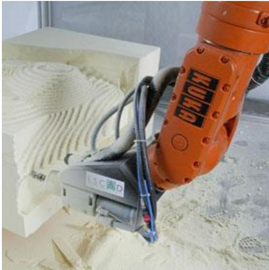
**KUKA CAD Driven Milling**
