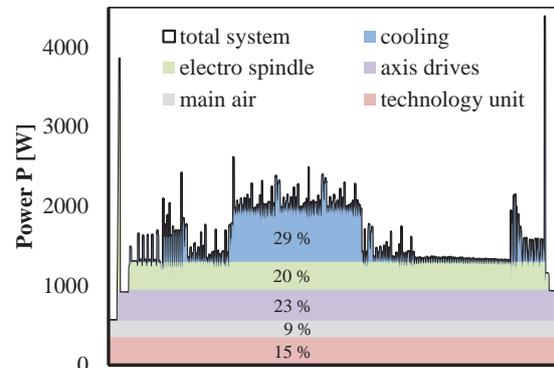
Fig. 6. Power profile milling test
