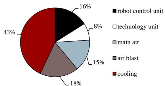
Fig. 1. Standby power consumption of the components
